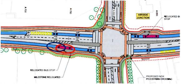
Extract from General Arrangement Drawing No BCIDB-JAC-GEO\_GA-0002\_XX\_00-DR-CR-0003 (red circle marks current location of proposed bus stop, navy circle is indicative revised position if this sufficient to avoid reposition of milestone)
